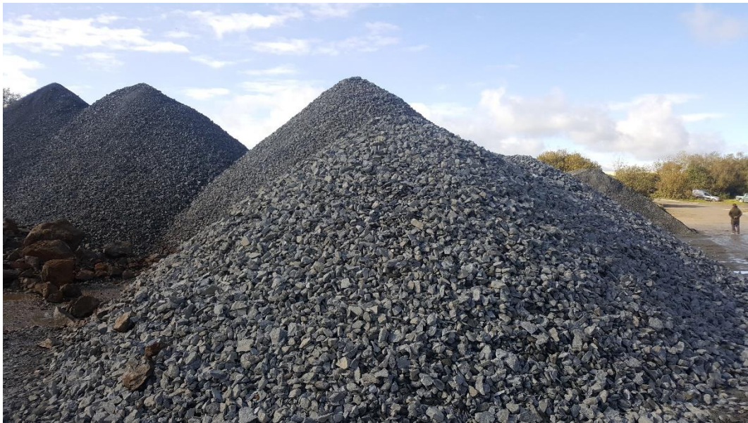
Figure 5. Crushed aggregate, produced from greywacke, Lower Quarry
